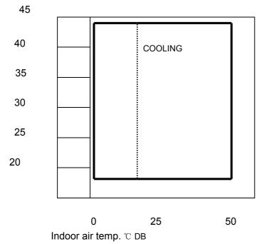
Note : The chart is the result from the continuous operation under constant air temperature conditions. However, excludes the initial pull-down stage.
